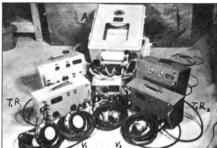
FIGURE 8 Echo-sounder used in experiment. (A : Indicator, T_1R_1 : 200 kc Transmitter and Receiver); T_2R_2 : 100 kc Transmitter; V_1 : 200 kc Transducers; V_2 : 100 kc Transducers.
