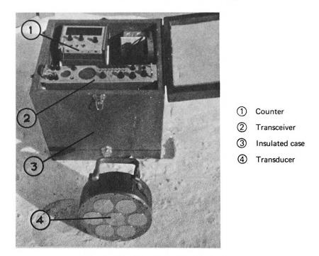
FIG. 2. — Equipment and carrying case.
