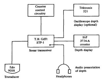
FIG. 1. -- Sounding System Block Diagram.
