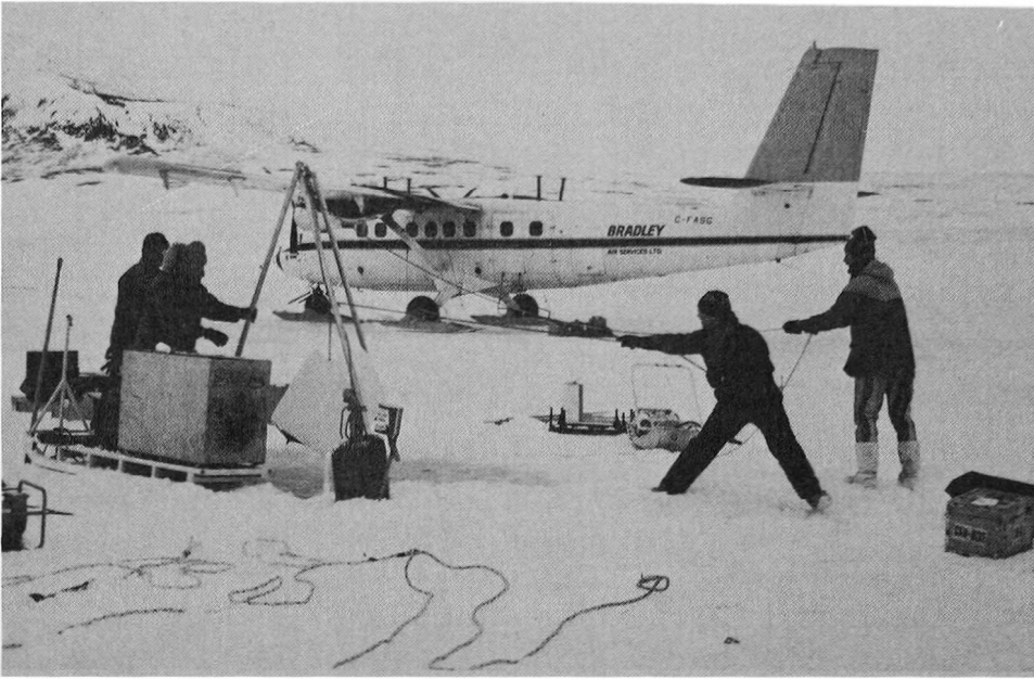
FIG. 6. — Removing ice cylinder to create 75 cm hole. After the ring is melted through the ice a rope is used to lift the ice cylinder out of the hole. The Twin-Otter in the background is the most common type of fixed-wing aircraft used on these types of surveys.
