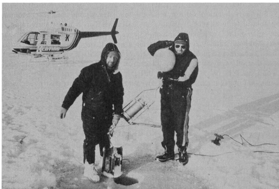
FIG. 4. — Temporary through-ice tide gauge mooring about to be deployed. Both helicopters and fixed-wing aircraft are used during these surveys.
