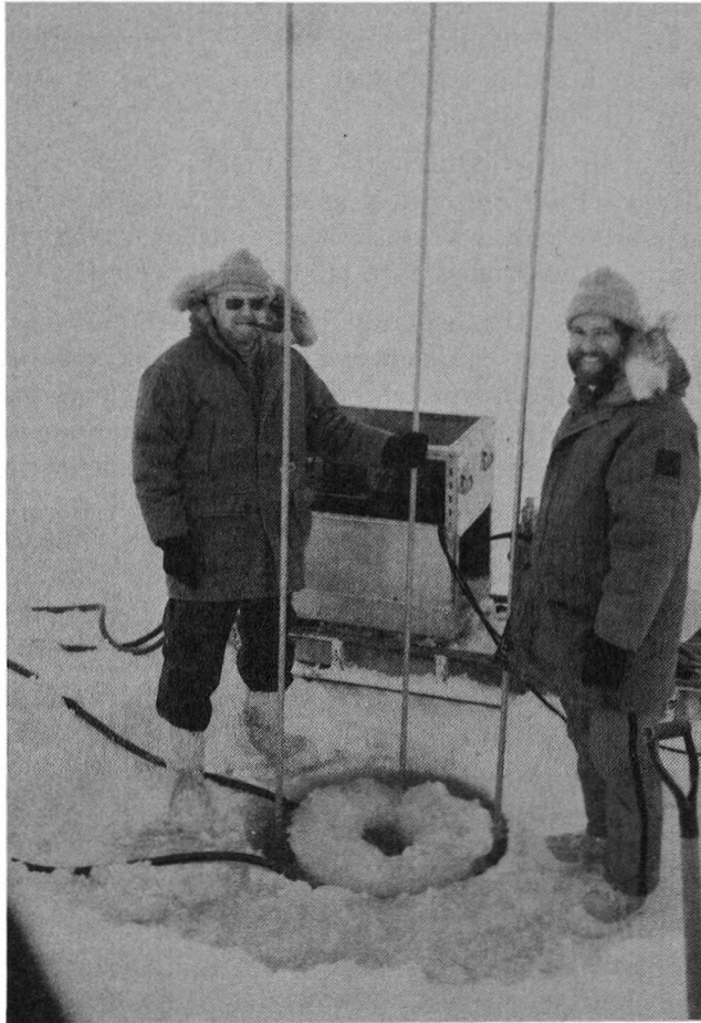
FIG. 5. — Ice hole melter in operation. Initially a 30 cm hole is drilled through the ice using a gasoline-powered auger. A 75 cm ring is then melted around the hole as shown. The hole melter consists of a circular pipe or melting ring with three rods attached for recovery. Water is heated in the furnace shown at the rear and is pumped through hoses to the melting ring.
