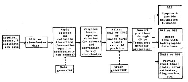
FIG. 1.- Block diagram of basic positioning system functions
