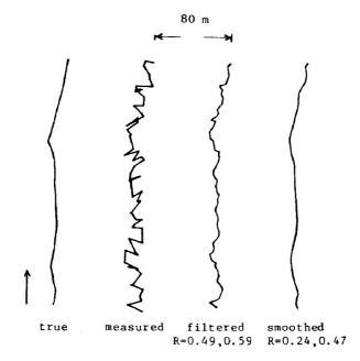
FIG. 7.— Example performance of the filter and smoother for 5-m measurement noise,  $0.5 \text{ m/s}^2$  process noise, and  $\sigma_a = 0.5 \text{ m/s}^2$ ; no heading, speed.
