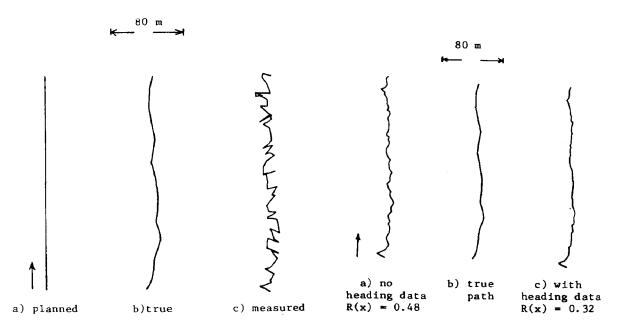
FIG. 3.— Track simulator output paths.
