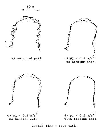
FIG. 5.- Filter output for 50-m radius U-turn at 5 m/s.
