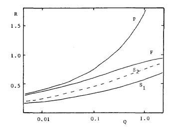
$\label{eq:Figure} \begin{array}{l} Fig. 2.- Noise reduction factors for predictor (P), filter (F), Houtenbos smoother (S_1), \\ & \mbox{and bidirectional smoother } (S_2). \end{array}$
