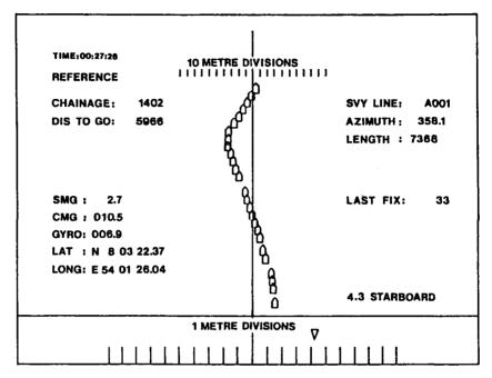
FIG. 4. - Left/Right Indicator Display.
