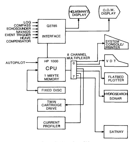
FIG. 2. — Data Logging System (DLS).
