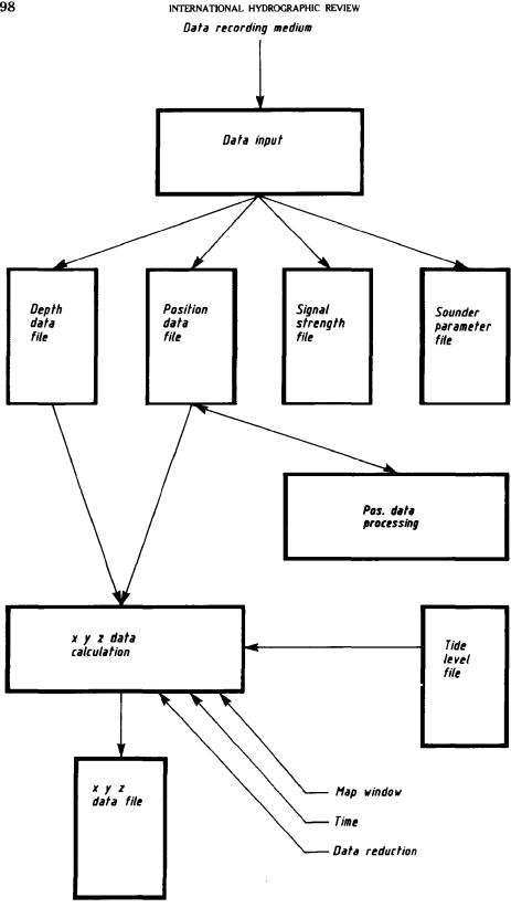
FIG. 3. - Simrad conversion module for EM100 (SC100).
