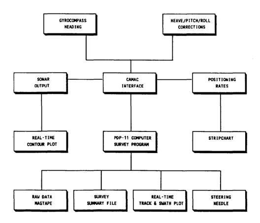
FIG. 2. - Shipboard Data Acquisition System.
