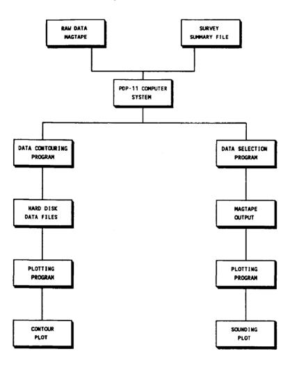
FIG. 3. - Shipboard Data Processing System.
