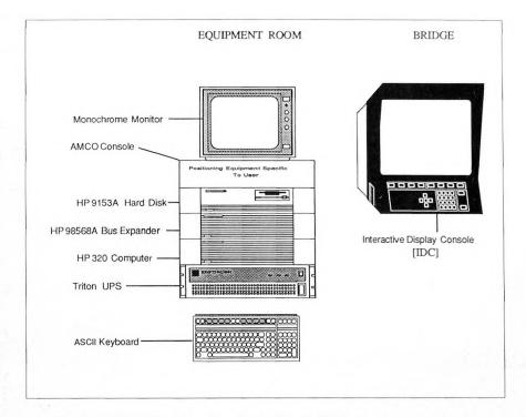
FIG. 1.- PINS 9000 - Interactive Display Console (IDC) and main equipment rack.
