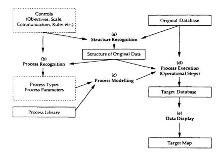
FIG. 2.- BRASSEL and WEIBEL model of generalization (after BRASSEL and WEIBEL 1988).
