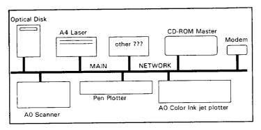
FIG. 2 - Shared peripheral devices.
