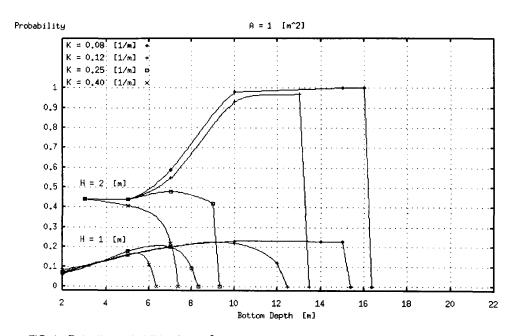
FIG. 1.- Detection probabilities for 1-m<sup>2</sup> circular cylinders in various water clarities, for 1-m and 2-m target heights, using a 20° scanner nadir angle on a 4m x 4m sounding grid.
