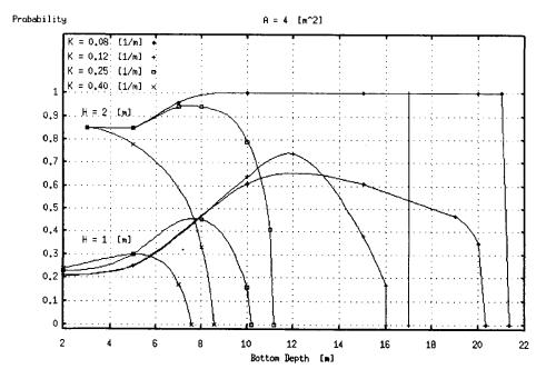
FIG. 2. Detection probabilities for 4-m<sup>2</sup> circular cylinders in various water clarities, for 1-m and 2-m target heights, using a 20° scanner nadir angle on a 4m x 4m sounding grid.
