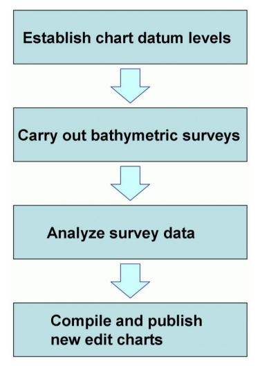
Figure 13 The flowchart of work for new edition nautical charts.
