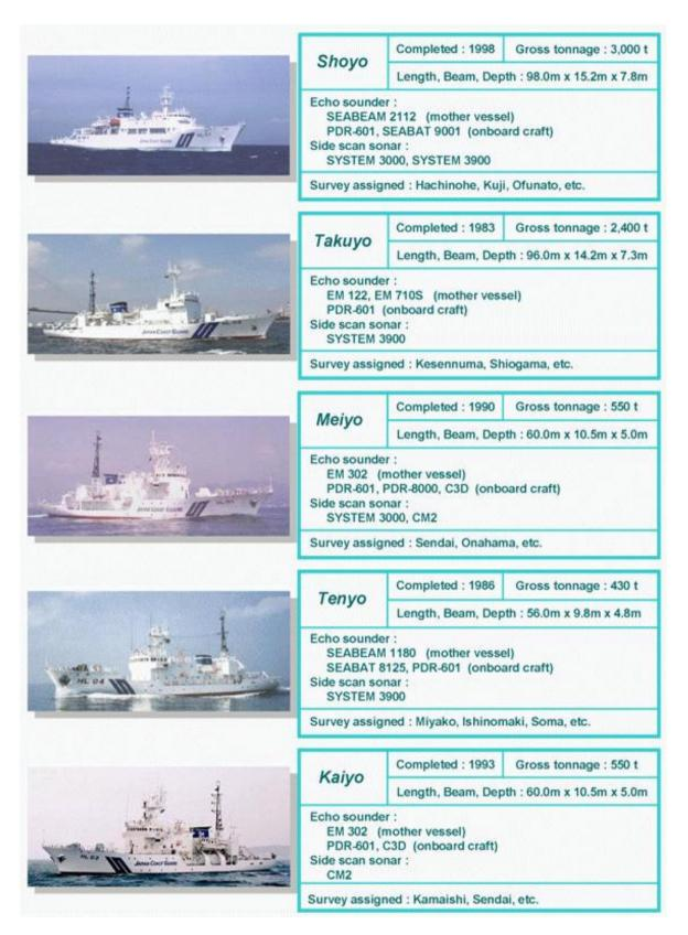
Figure 2 Specifications of the dispatched survey vessels.
