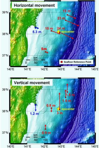
Horizontal (upper panel) and vertical (lower carried out the Figure 10 panel) displacement at the seafloor reference points and (Figure 11) along natural coastlines n June 2011. the GPS station, associated with the earthquake. Red squares and blue dots show locations of seafloor reference points and the GPS station respectively.
