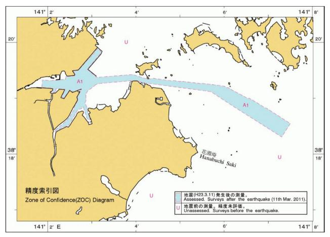
Figure 16 The Zone of Confidence (ZOC) diagram newly introduced in a new edition nautical chart of Shiogama Section.
