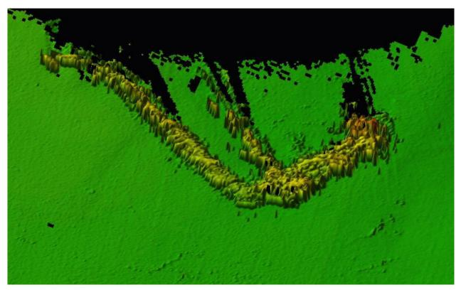
*Figure 8* The multibeam echo sounder record of a fallen crane from a quay.
