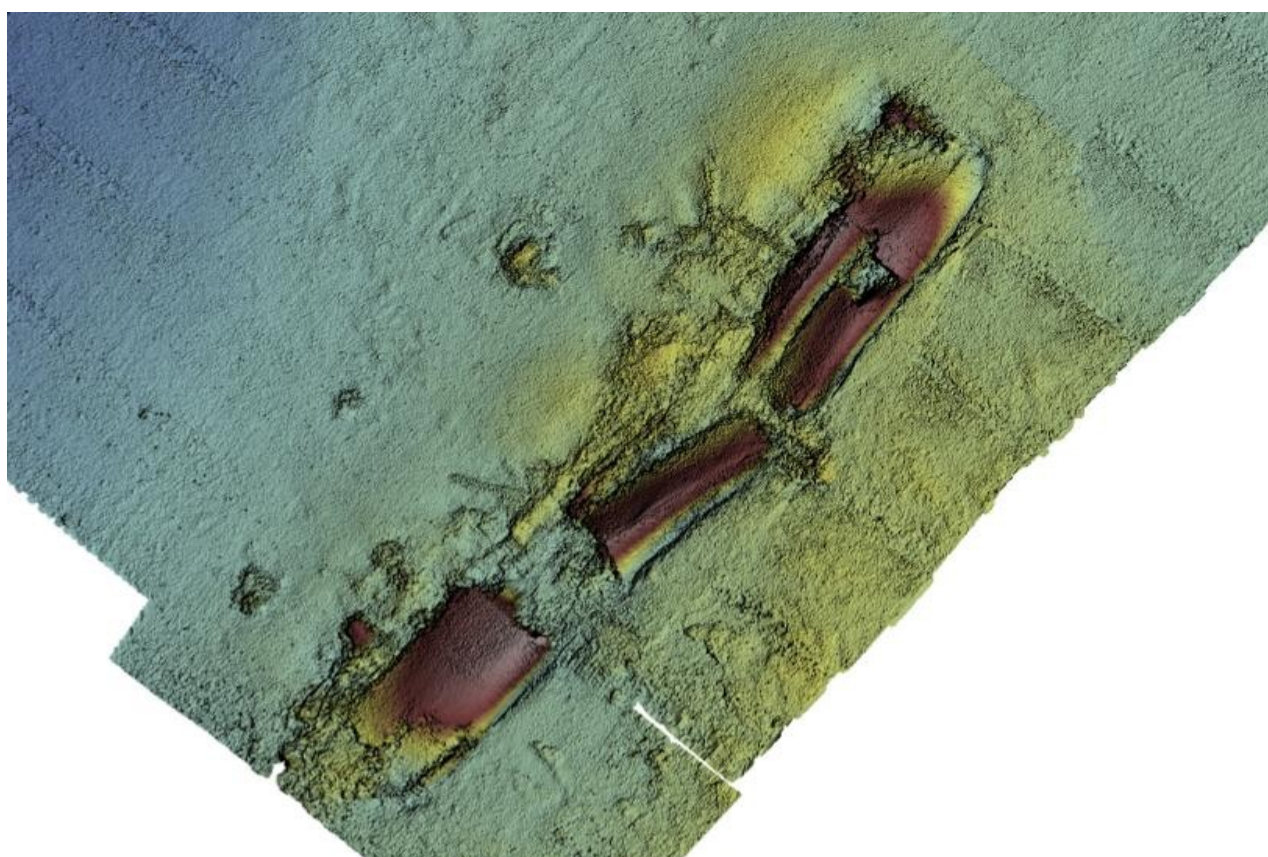
Figure 2: Bathymetry of the wreck of the SS Shirvan, 100m bow to stern. Collected using a GeoSwath 500kHz sonar on a Gavia AUV in ~100m water depth. The data was processed to a 20cm xyz grid in OIC CleanSweep3 using interferometer-appropriate data processing techniques and Simultaneous Localisation and Mapping (SLAM) AUV navigation corrections.
