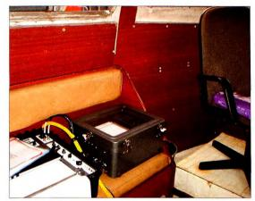
Photo 2: Odom Hydrotrac Echosounder onboard survey Boat. (Photo Courtesy: Innocent Egbuh).
