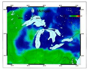
Figure 6: Michigan zenith wet delay (in cm) for July 11, 2004. Image derived from the NOAA troposphere zenith delay maps. The red square delimits the test area.
