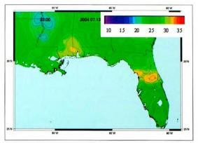
Figure 23: South East zenith wet delay (in cm) for July 13, 2004
