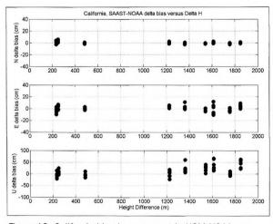
Figure 19: California bias improvement in USM NOAA over USM SAAST versus height difference.
