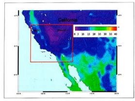
Figure 12: California zenith wet delay (in cm) for July 11, 2004
