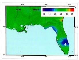
Figure 22: South East zenith wet delay (in cm) for July 11, 2004
