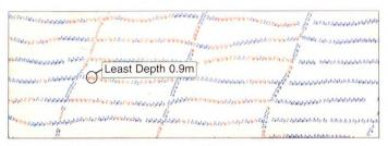
Figure 9 - Acoustic survey across boulder bed.
