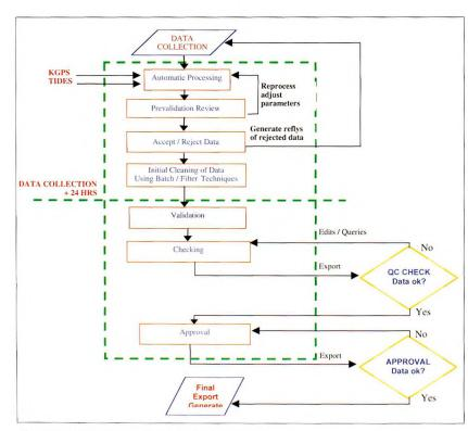
Figure 5 – LADS Data processing flow diagram.
