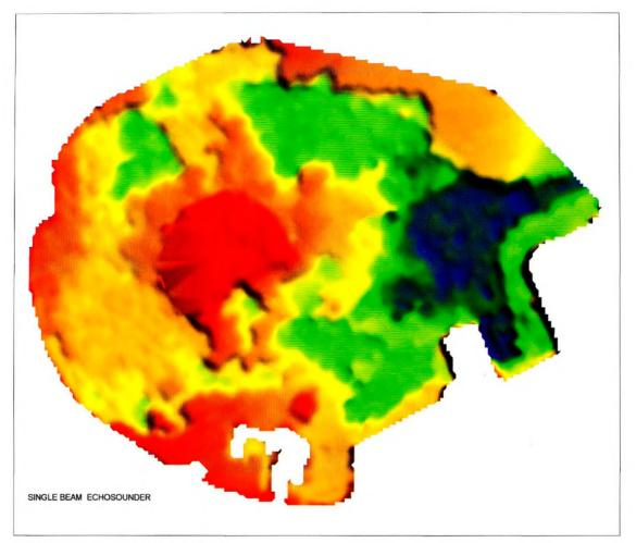
Figure 6: Image from single beam survey
