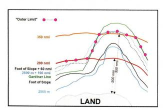
Figure 3: Article 76 main features and their combinations that need to be determined and the combination of them in order to derive the 'Outer Limit'. This illustration is not to scale [Modified after Smith and Taft, 2000]
