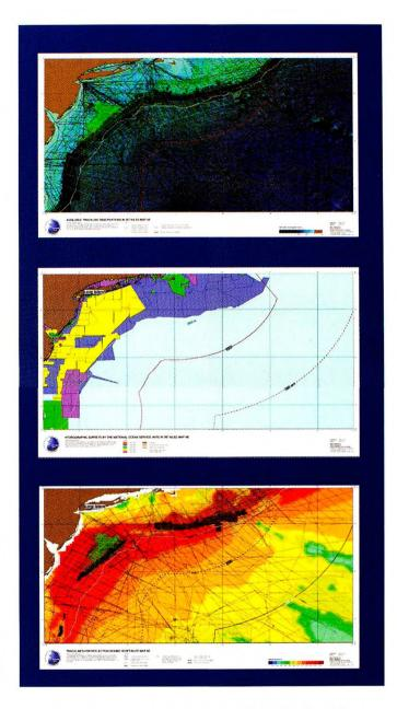
Figure 6: Detailed maps of area NE (see Figure 1) showing various combinations of all available trackline data in the area. The maps are shown in reduced scale from Jakobsson et al. [2002]. A: Tracklines color coded by source and overlain on a shaded relief representing ETOPO2; B: Available high-density NOS data in the NE area; C: Distribution of seismic reflection profile data overlain on sediment thickness information from NGDC
