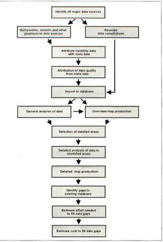
Figure 4: Flowchart illustrating the general work plan and approach designed for the evaluation of content and condition of existing relevant data holdings in all areas where the U.S. may have a potential claim for extension of the continental shelf beyond the present 200 nautical mile limit
