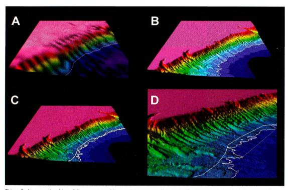
Figure 9: An example of how full-coverage multibeam data can result in a significant extension of a claim beyond the claim that could have been made based on single beam sonar data.
