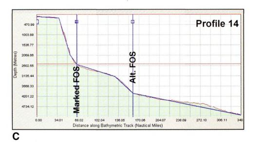
Figure 7 C: Bathymetric profiles 9 and 14 in detailed study area NE. The locations of these profiles are shown in A and B. The ambiguity in location of the FOS is clearly illustrated. The 'Marked FOS' is the location marked with a dot in A and B. Alternative locations for the FOS are shown in each profile. Note that the vertical exaggeration in the bathymetric profile accentuates gradient changes
