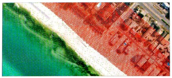
Figure 1a: Fusion of hydrographic and topographic lidar data with imagery: data points
