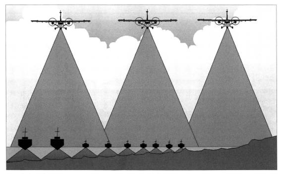
Figure 4: Depiction of lidar and multibeam sonar operation in shallow water
