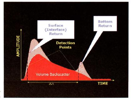
Figure 2: Schematic lidar waveform with key elements
