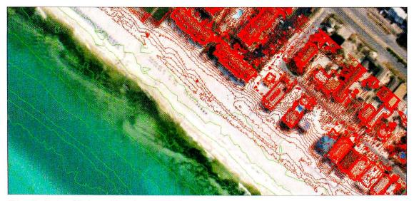
Figure 1b: Fusion of hydrographic and topographic lidar data with imagery: elevation contours
