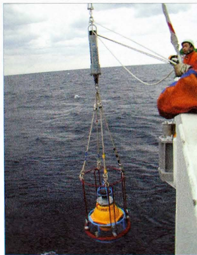
Figure 8: Photo of a precise transponder of JHD to use GPS/Acoustic positioning just before the placement on the sea floor
