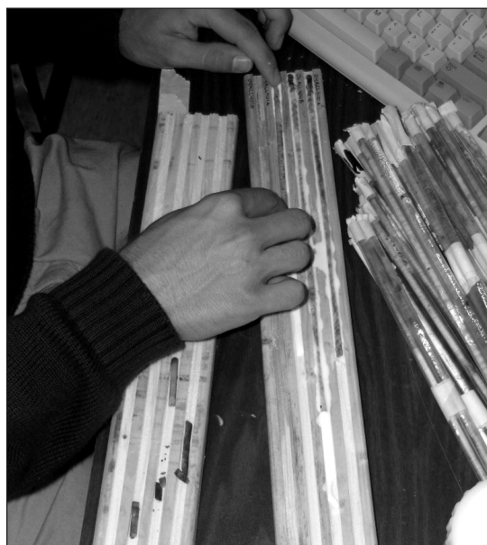
Fig. 5 Slotted mounting boards are used to hold the increment cores for preparation and sanding. Labels delineating each core are transferred from the field to the boards so the specific location of each core can be tracked.
