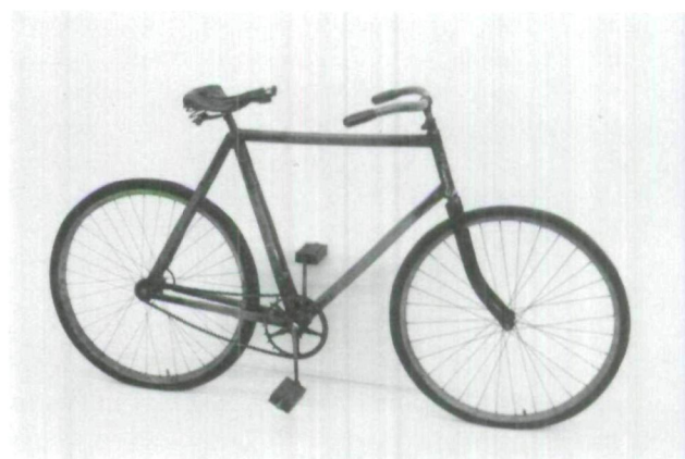
Fig. 1. Comet bicycle, Comet Cycle Company, Toronto, ca. 1895. The bicycle has a wooden frame with metal components and pneumatic tires. The Comet Cycle Company, a partnership of Thomas Fane (manufacturer of the bicycle in figure 2) and Charles Lavendar, produced metal bicycles as well. (Photo: National Museum of Science and Technology (N.M.S.T.), cat. no. 760670.)
