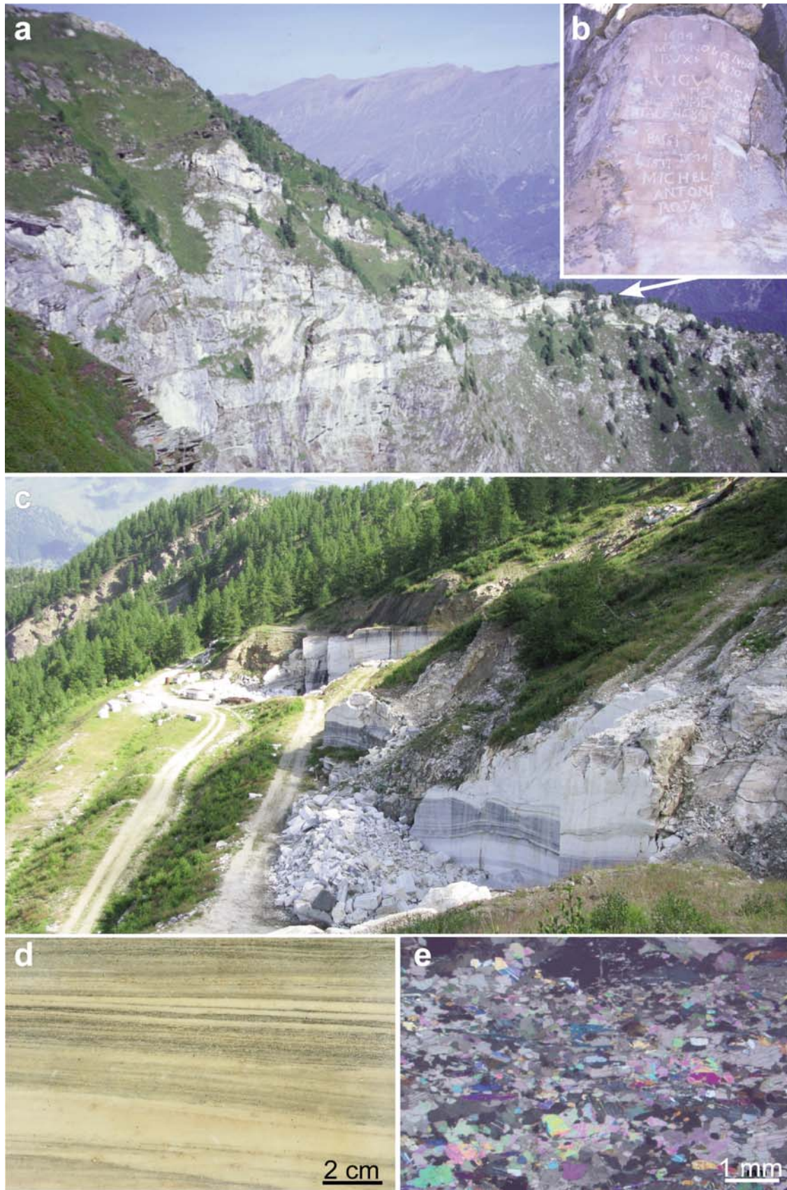
Figure 10. a) The eastern slope of the Rocca Bianca Mount (Germanasca Valley), where traces of the historic quarry of Prali Marble are still visible (quarry site 12 in Figure 2); b) graffiti dating back to the end of 1500 carved on a quarry face; c) Maiera Quarry, located along the western slope of the Rocca Bianca Mount (quarry site 11 in Figure 2), where the marble was exploited as recently as 2005; d) macroscopic aspect of the marble, characterized by regular intercalation of carbonate (light) and phyllosilicate layers; e) microscopic aspect (crossed-polarized light), marked by oriented crystals of tremolite and white mica, which define the anisotropy of the rock. Photo credits a) and b): Alessandro Ghelli and Cadoppi et al. 2008, respectively.
