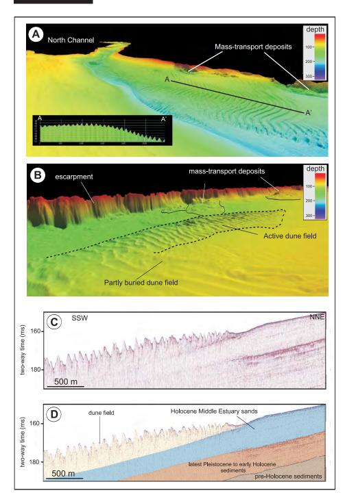
**Figure 6.** A. Perspective view toward the south showing an 8.5-km-long dune field characterized by curvilinear crests. B. Perspective view toward the north showing a 7-km-long dune field. C and D. Very high-resolution seismic profile and interpretation illustrating a dune field within the St. Lawrence Middle Estuary. See Figure 2A for locations.
