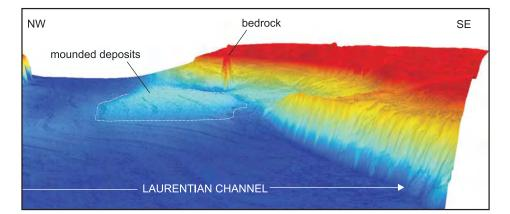
**Figure 3.** Perspective view toward the north showing mounded deposits in the Laurentian Channel, southwest of Rimouski. See Figure 2A for location. This large-scale geomorphological feature is interpreted as being shaped by strong bottom currents. The width of the near view is about 9 km.
