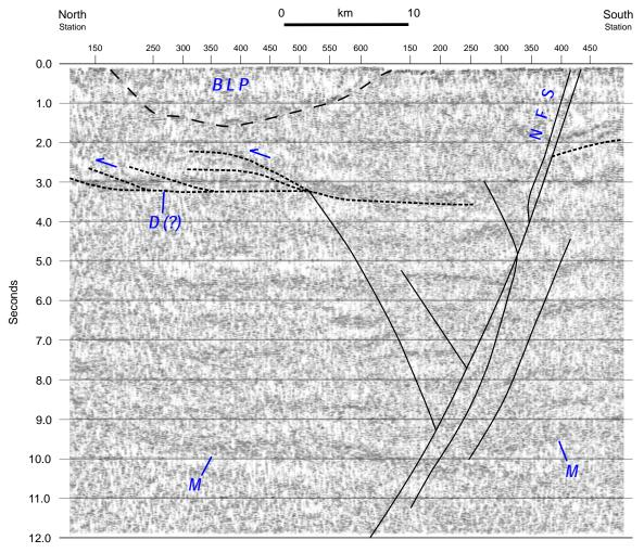
**Figure 9.** Upper part of Bottle Lake seismic reflection profile. Vertical scale is two-way travel time in seconds. Gently east-dipping reflectors beneath the Bottle Lake pluton (BLP) at 2 to 3 seconds depth are interpreted as northwest-directed blind thrusts above a possible decollement (D). M = Moho; NFS = Norumbega fault system (Waite fault zone). (Modified from Costain *et al.* 1989).
