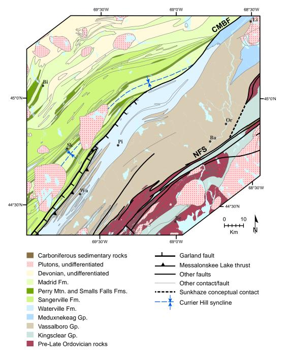
Figure 11. Proposed connection of Messalonskee Lake and Central Maine boundary faults. Compare with Figure 4. Sunkhaze conceptual fault separates sandstones of the Vassalboro and Kingsclear groups east of Orono in an area with little outcrop control. Modified after Osberg *et al.* (1985); Osberg (1988); Ludman (2010).
