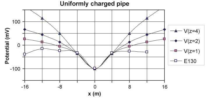
**Fig. 16.** Calculated potential on a traverse over a long pipe with uniform charge per unit length for 3 different burial depths, z. Corresponding surface charges are (assuming radius R=0.9 m): -0.45 (z = 1 m), 0.79, and 1.84 pC/m<sup>2</sup>. Reference distances r<sub>0</sub> are 9, 7, and 6.85 m, respectively. Also shown is measured profile E130 over the storm sewer.
