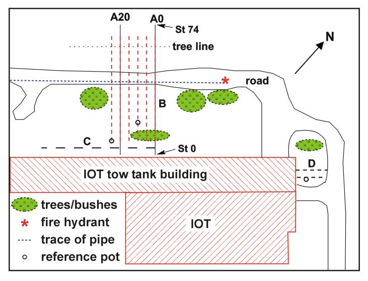
**Fig. 1.** Sketch of survey grids and lines A, B, C, and D in Survey Area I, northwest of IOT building. The tow tank building is 236 m long: about two thirds of that length is shown. Main survey lines are spaced at 5 m intervals. Lines A0 and A20 are 20 m apart. Station spacing is indicated by length of dashes and spaces. The reference pot between lines A0 and A20 was used for surveys A and C.
