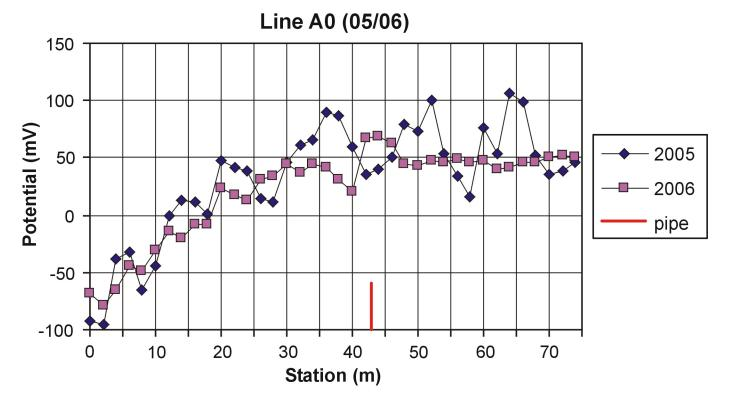
**Fig. 19.** Comparison of profiles along Line A0 on August 18<sup>th</sup> and 22<sup>nd</sup>, 2005, during dry, warm weather, and June 2<sup>nd</sup> and 5<sup>th</sup>, 2006, when the weather was cool and damp.
