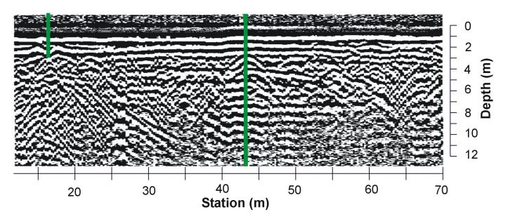
Fig. 4. GPR profile of line A0 (Fig. 1) taken Oct 4, 2005. A refraction hyperbole due to the water pipe shows clearly at station 44.
