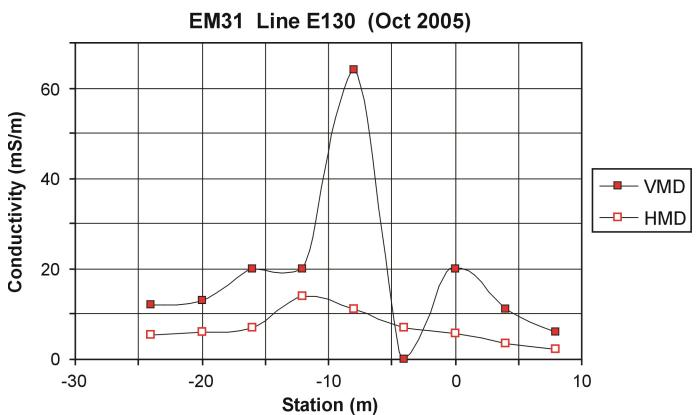
Fig. 14. Ground conductivity profiles taken using the Geonics EM31 held at hip level on Line E130.
