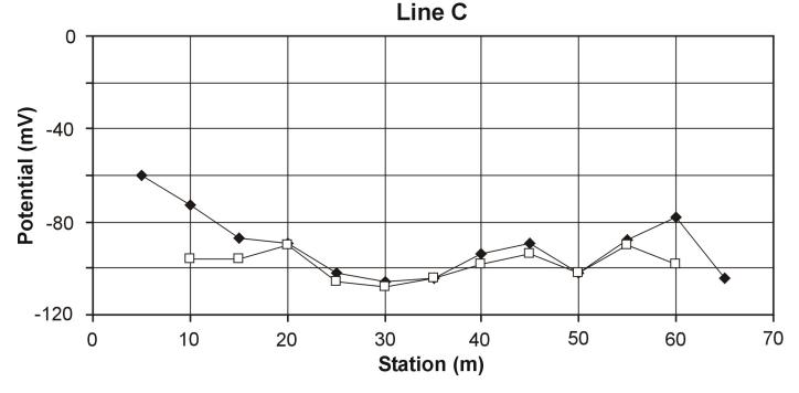
**Fig. 10.** SP profile along Line C, parallel to the IOT building at a distance of 5.4 m, along station number 4 of Grids A and B. Station 0 is on Line A0, and Station 20 is on Line A20. Closed symbols are for a traverse in ascending station numbers. Open symbols indicate a return traverse in the opposite direction.
