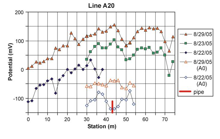
**Fig. 6.** SP profiles of line A20 (Fig. 1) taken on 3 different days in August, 2005. Potential values apply to profile 8/22/05. Profiles 8/23/05 and 8/29/05 are offset by 50 and 100 mV respectively. Also shown are two profiles over the water pipe on line A0. Profiles 8/29/05(A0) and 8/22/05(A0) are offset by -100 mV and -170 mV, respectively.
