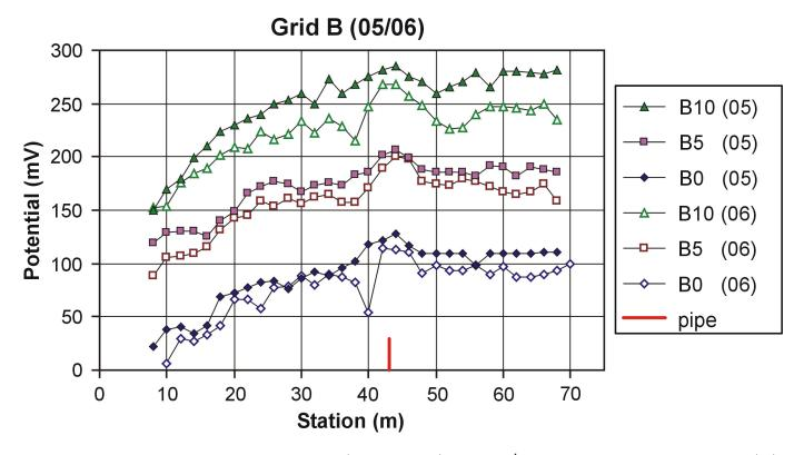
**Fig. 20.** Profiles in Grid B taken on September 2005 (closed symbols) and June 5<sup>th</sup>, 2006. 2005 profiles are offset from B0(05) by 75 mV, 2006 profiles by 85 (B0-B5), and 75 mV (B5-B10). B0 (06) is subset of Line A0 (2006) in Fig. 19. B0 (05) may be offset 2 m relative to B0 (06).
