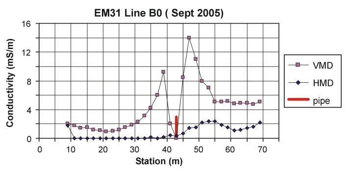
**Fig. 5.** Ground conductivity profiles taken using the Geonics EM31 held at hip level. The median penetration depth below the surface is about 2.4 m in the VMD configuration, and 0.6 m in the HMD configuration.
