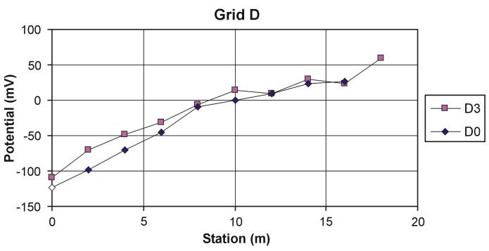
Fig. 11. SP profiles of lines D0 and D3 (Fig. 1), measured on October 2, 2005.
