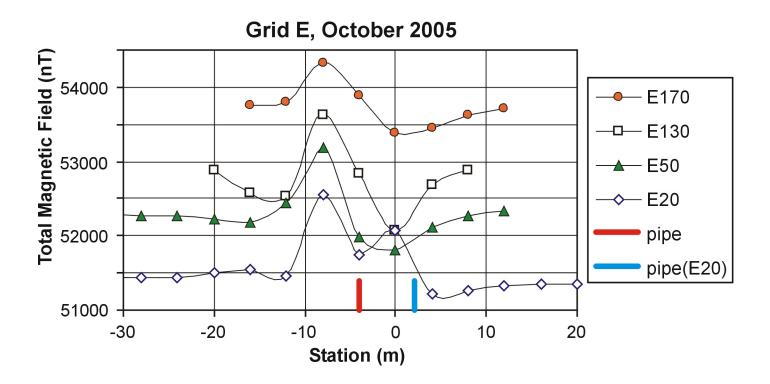
Fig. 15. Profiles of total magnetic field on selected lines of Grid E, October, 2005. For ease of viewing, successive profiles are offset by 800 nT.
