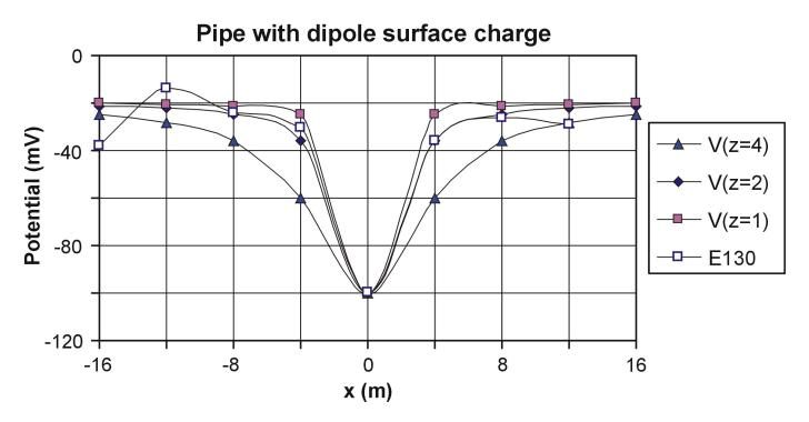
Fig 17. Calculated potential on a traverse over a long pipe with cosine surface charge (Eqn (2)) for 3 different burial depths, z. Corresponding values for  $\sigma_0$  are (assuming radius R=0.9 m): -0.875 (z=1 m), -1.75, and -3.5 pC/m<sup>2</sup>. Potential offset V<sub>0</sub> is 20 mV. Also shown is measured profile E130 over the storm sewer.
