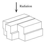
Fig. 3. The special design of the leaves of the MLC which leads to the tongue-and-groove constraint.
