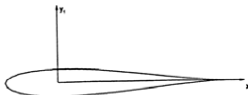
Figure 4. Schematic of a Joukowski Airfoil
