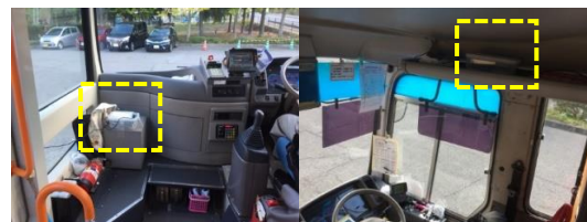
Fig. 3. Installing WiFi Scanner on Bus No.1 And Bus No.2
