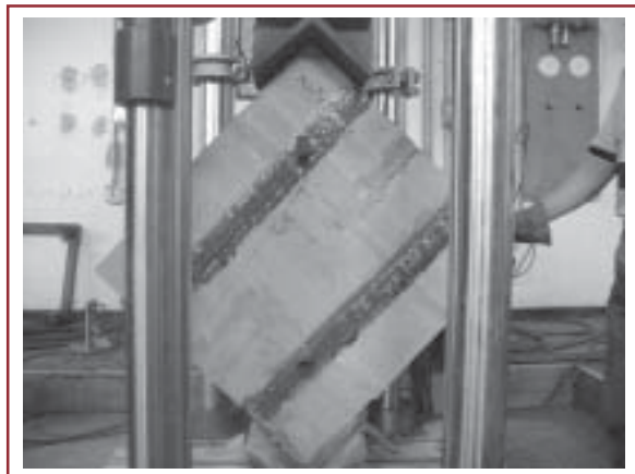
Figure 3. GFRP Strengthened wallettes subjected to diagonal tension.
