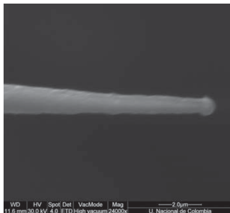
Figure 8. SEM image of the tip-radius obtained with 3mm of immersion.
