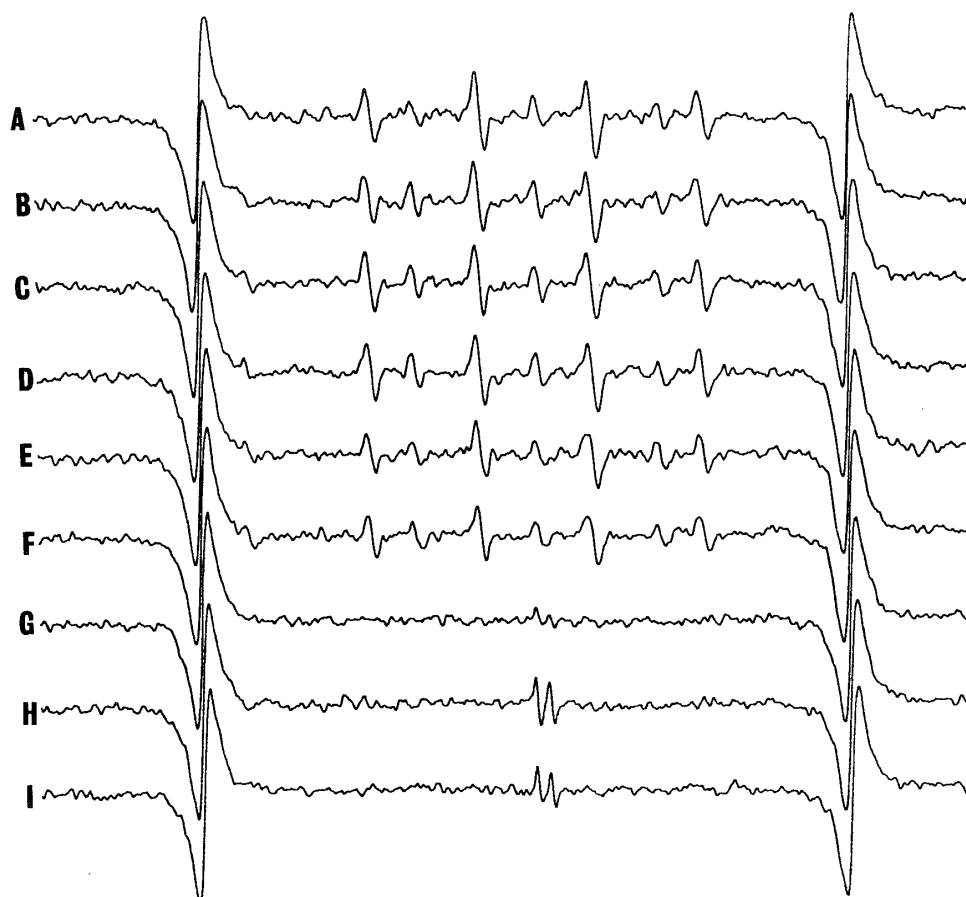
Fig. 2 ESR spectra obtained from the irradiated human serum at various ascorbic acid concentrations.
