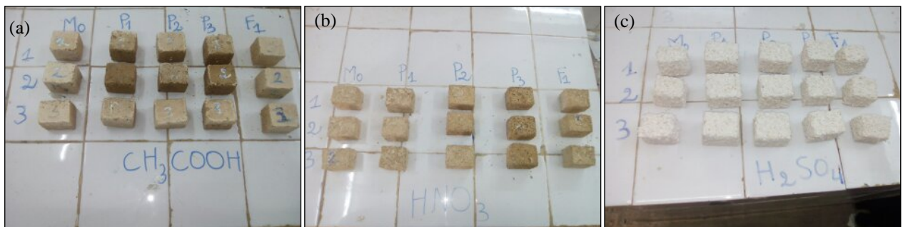
Fig. 16- State of the specimens after immersion for 28 days in the various acids.
