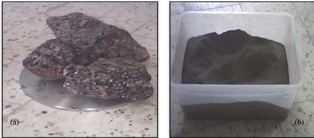
Fig. 1 – (a) Natural pozzolan slag before grinding; (b) natural pozzolan powder after grinding.
