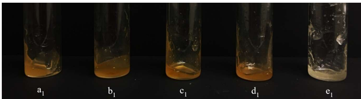
Figure 5.15. Solid resin (1 g) samples in glass vials: (a 1 ) PPO192/Gly PU; (b 1 ) PEO200/Gly PU; (c 1 ) PPO192 PU; (d 1 ) PEO200 PU; (e 1 ) PPO192/Trigly PU.
