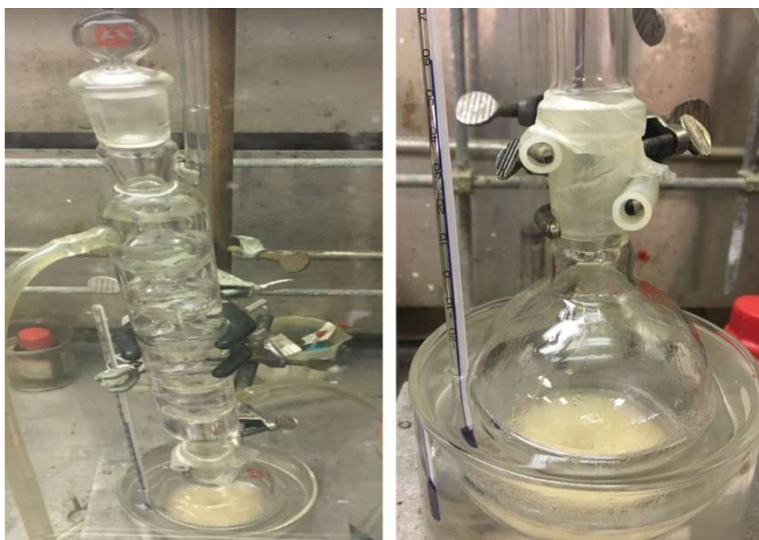
Figure 2.1. Reaction setup for HUTEAB synthesis. White precipitated reaction product can be seen at 60° C.
