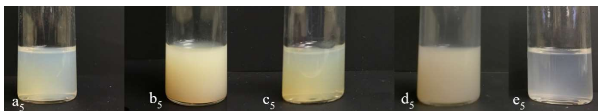
Figure 5.19. Dispersions of Fig. 5.18 after 10 minutes of sonication: (a 5 ) PPO192/Gly PUD; (b 5 ) PEO200/Gly PUD; (c 5 ) PPO192 PUD; (d 5 ) PEO200 PUD (stirred for 1 minute); (e 5 ) PPO192/Trigly PUD.
