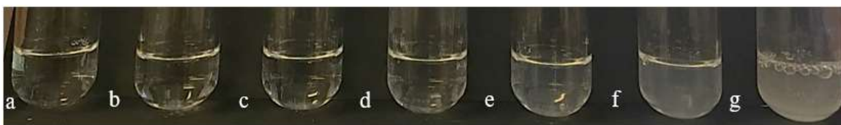
Figure 5.34. After 1 hour of addition of 2.25 ml KI solution of concentration, \log([KI]/M) : (a) -5; (b) -4; (c) -3; (d) -2.25; (e) -2; (f) -1.75; (g) -1 in 0.25 ml of 0.5% PPO192/Trigly PUD.
