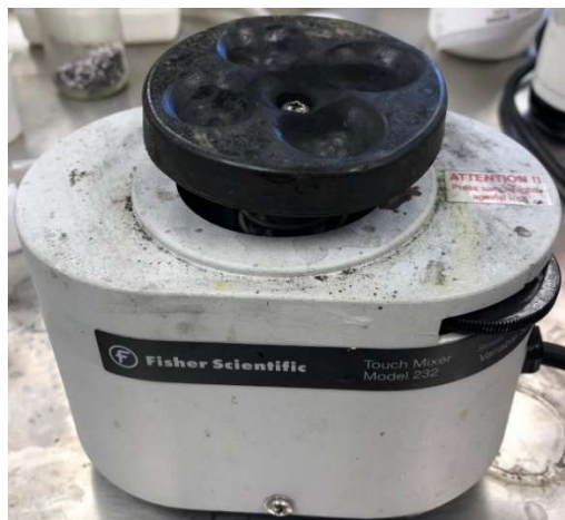
Figure A.2.1 Fisher Scientific vibratory Stirrer used to stir samples in this thesis work.
