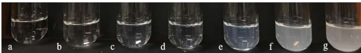
Figure 5.32. After 1 hour of addition of 2.25 ml NaBr solution of concentration, \log([\text{NaBr}]/M) : (a) -3; (b) -2; (c) -1.5; (d) -1.4; (e) -1.3; (f) -1.2; (g) -1.1 in 0.25ml of 0.5% PPO192/Trigly PUD.
