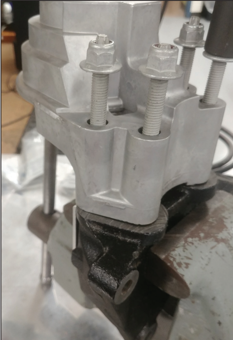
Figure 2. Die Cast Aluminum Joint: The image above represents the initial test set up
