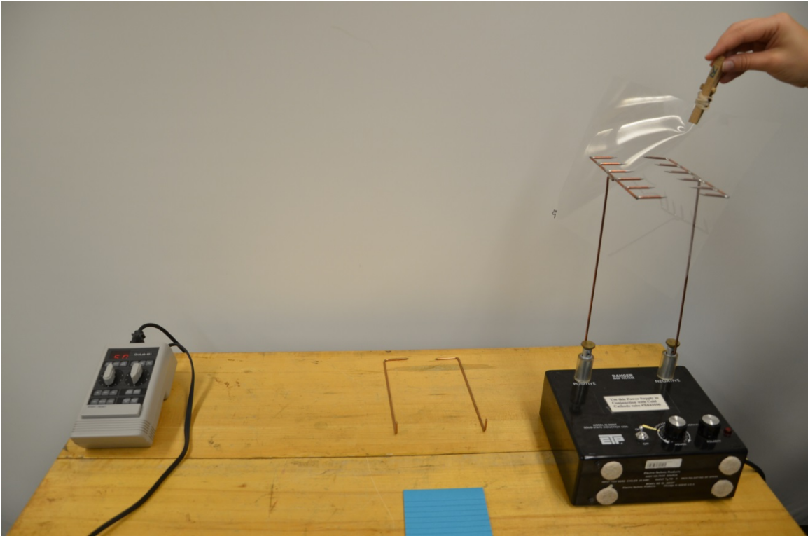
Figure 8: Photograph of the solid-state induction coil power supply, made by Electro-Technic Products Model ID-300ST, charging station. The induction coil has a multi-needlepoint discharge probe attached to each output terminal. It takes 115 V, 50/60 cycle input and converts it into a 3–5 cm pulsating dc spark that is connected to a GraLab Model 451 timer.
