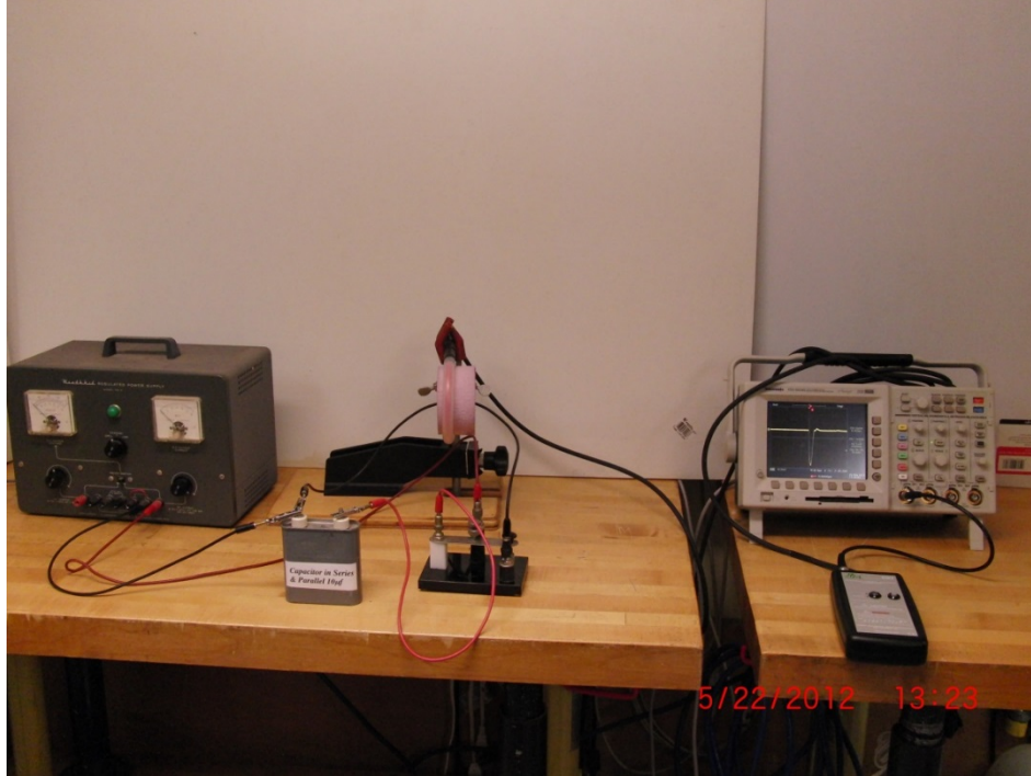
Figure 25: Photograph of the control situation setup to test the Rogowski coil using a 10 \mu\text{F} capacitor.
