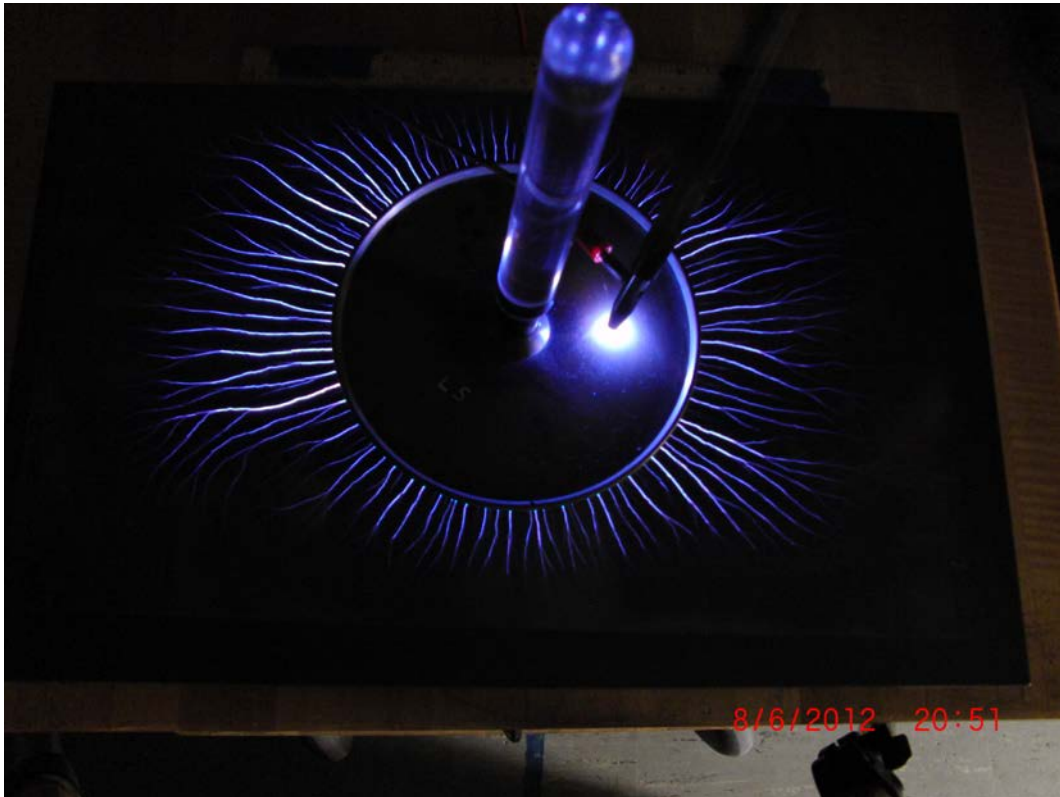
Figure 29: Photograph of an 11" x 17" dielectric sheet discharge from a 17 cm diameter flat, circular metal charge transfer plate.
