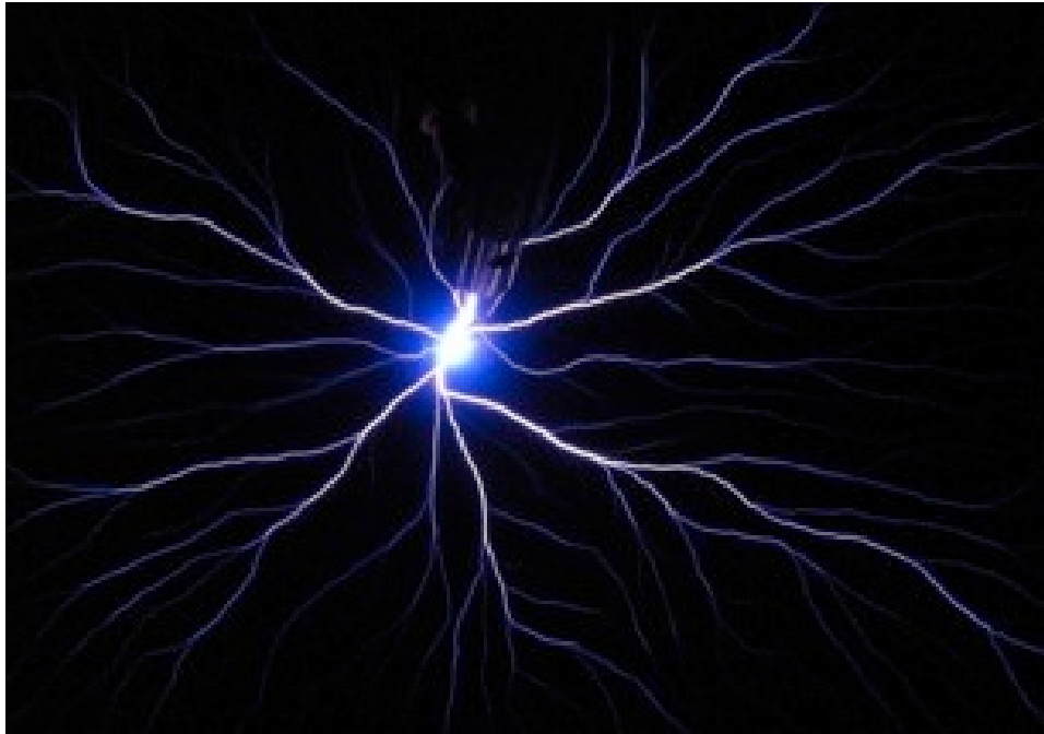
Figure 21: Photograph of a radial Lichtenberg discharge produced by an 8.5" x 11" dielectric sheet that was charged for 3 sec/side.
