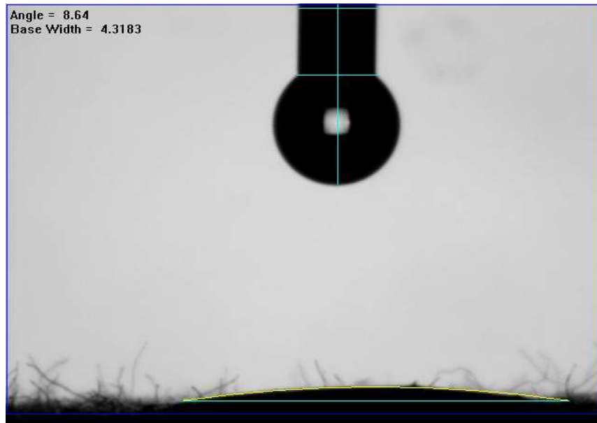
Figure 13. Contact angle reading for original uncoated sample showing one of the lowest contact angles: 8.64^\circ
