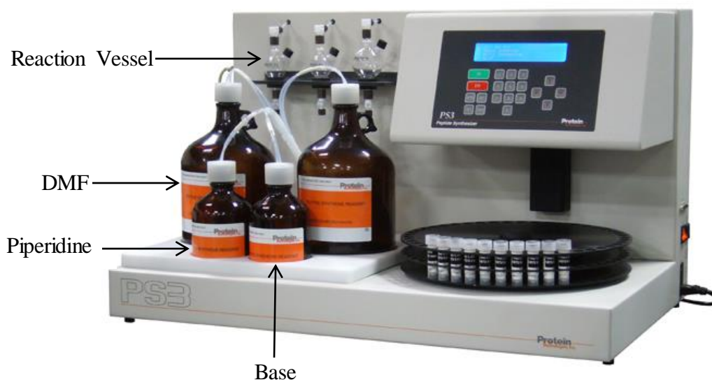
Figure 6: PS3 Peptide Synthesizer. Fmoc-amino acids mixed with activating agent are placed in the vials. Piperidine is the deprotecting agent and DMF (dimethylformamide) is the solvent.
