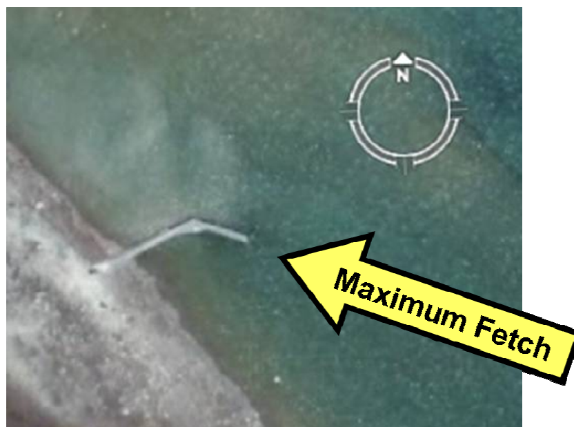
Figure 6. Crib dock with lakeward end angled to face anticipated ice load.
