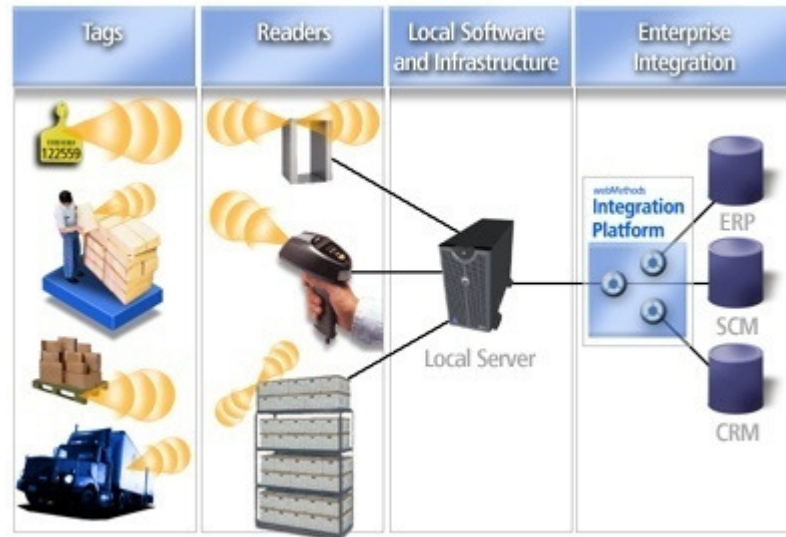
Figure 1. The Four Main Components of an RFID System
