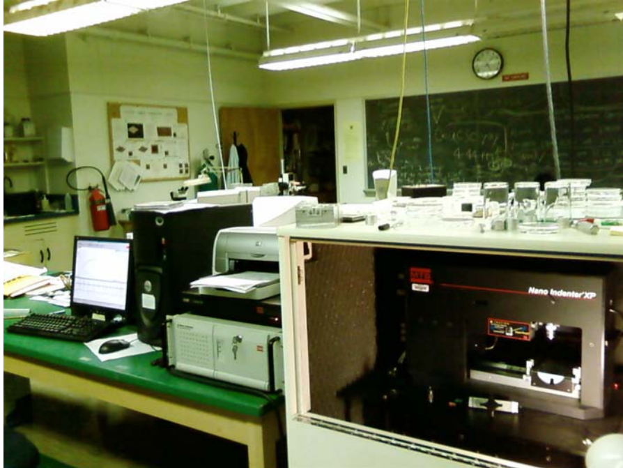
Figure 1: Nano indenter XP and CSM equipment in the Surface Science and Nanotribology Laboratory. It is operated using the attached computer.
