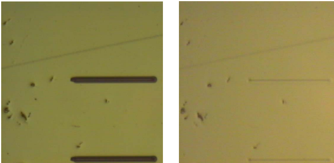
Figure 8: optical images of sample 1 that clearly shows the recovery due to heat treatment.
