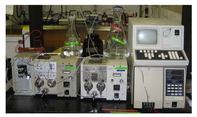
Figure 9. Waters 717 HPLC with 484 UV absorbance detector having Phenomenex Jupiter C18 column used for the separation of pure peptide using 0.1% TFA-water and 0.1% TFA-acetonitrile mobile phases.
