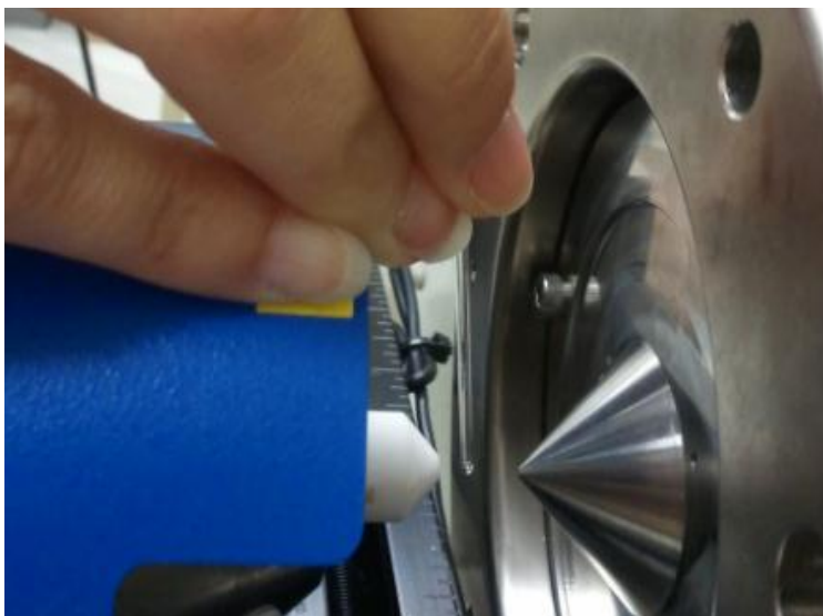
Figure 6. The DART ion source, showing the gap where samples are introduced.
