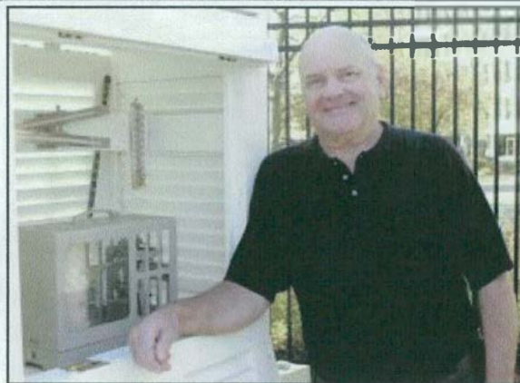
STATION MANAGER: Carl Ojala, professor of geography at EMU for 34 years, is officially retiring Aug. 1. Ojala stands next to a hydrothermograph, an instrument that measures temperature and relative humidity. Ojala has faithfully taken readings from the instrument, located outside Strong Hall, every day for the last 20 years.
