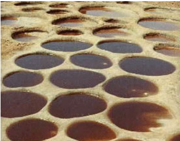
Figure 21: Portioning off the salt water into smaller bodies for the evaporation method of salt production. 135
