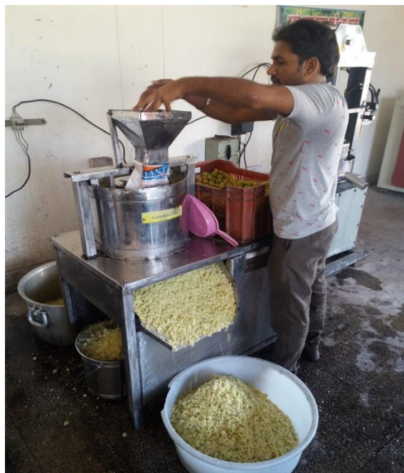
Figure 3. Aonla Shredding in Operation Performed by the Entrepreneur
