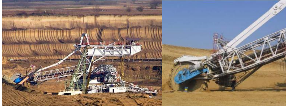
Fig.1. Type of Excavator SRs 1300 and working wheel
