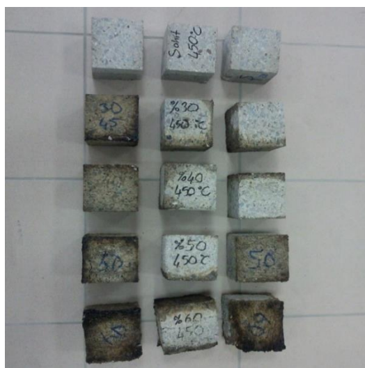
Fig. 11. The mixtures exposed to 450 °C
