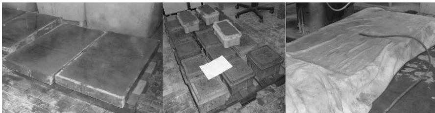
Figure 3. Manufacturing of the specimens; (left) casted slab; (middle) reference cube specimens; (right) slabs under wet towels.
