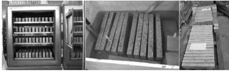
Figure 6 (left) Climatic chamber; (middle) Water immersion; (right) air exposure
