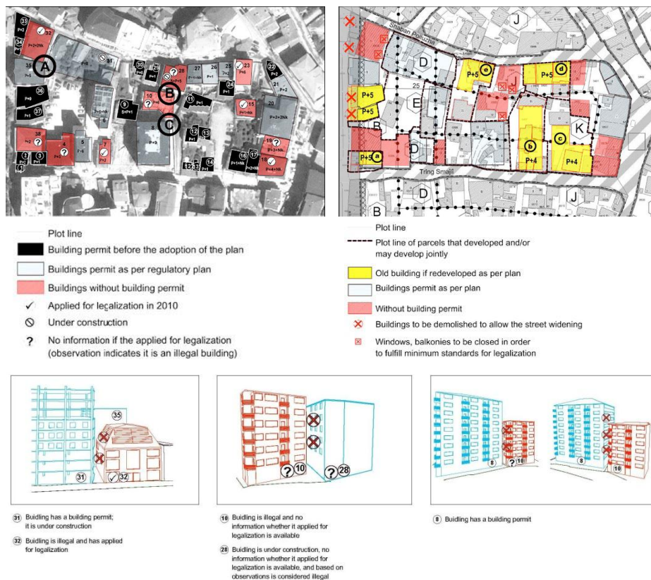
Figure 13. Case study Dodona (top left: map showing the status of buildings in October 2011 with regards to legalization; top right: map showing possible solution in implementing both, planning and legalization parameters; bottom: interpretation of minimum standards for legalization for identified problems)
